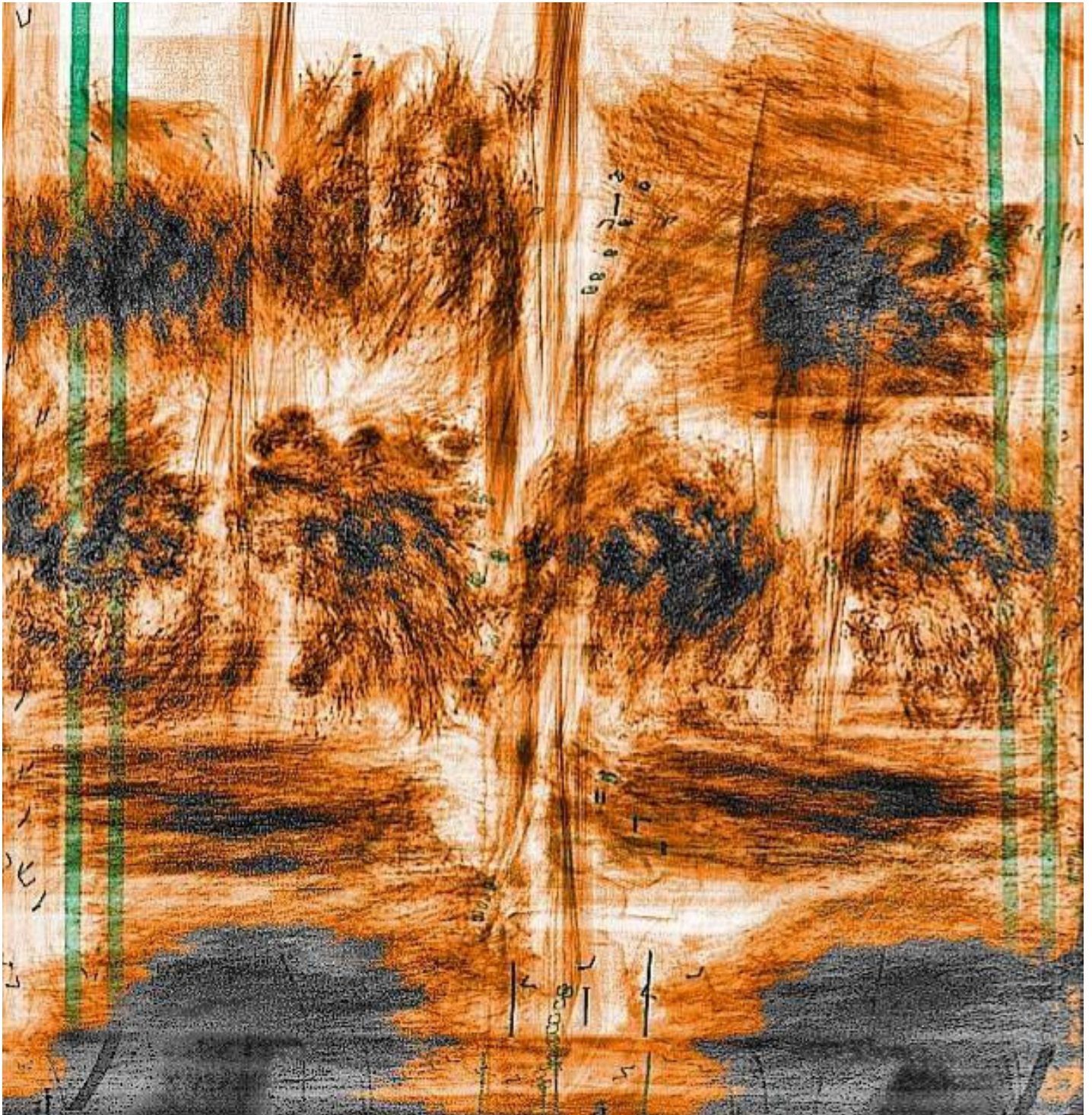
Typical x-ray image of Khat bundles with stalks clearly visible
